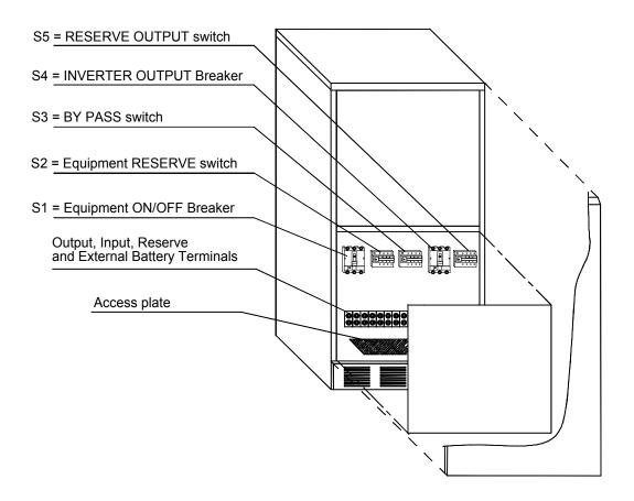
Figure 25 – 50/80kVA: Connections
